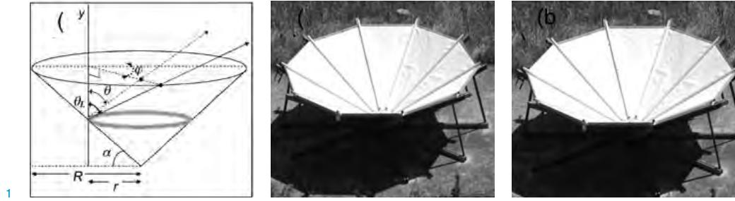
**Figure 1** Integration scheme for the funnel shape ( $0 < \theta < \theta_L$ ,  $0 < \phi < 360^\circ$  and  $0 < r < R$ ). (b) Photo of the funnel-shaped condenser ( $7.3 \text{ m}^2$  surface area with  $60^\circ$  cone angle,  $30^\circ$  from horizontal). The internal surface of the experimental condenser is coated with OPUR ([www.opur.fr](http://www.opur.fr)) low density polyethylene film insulated from below with 3 cm styrofoam.
