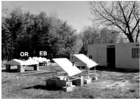
**Figure 7** "Egg Box" (EB) and "Origami" (OR) type condensers with the planar reference condenser (R). (T is an additional planar condenser).
